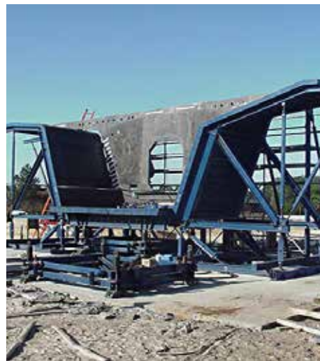
Pre-cast, segmental, short line casting machine designed for robust and speedy segmental bridge construction.
