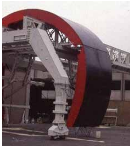
Custom hydraulic actuated tunnel forming system.
